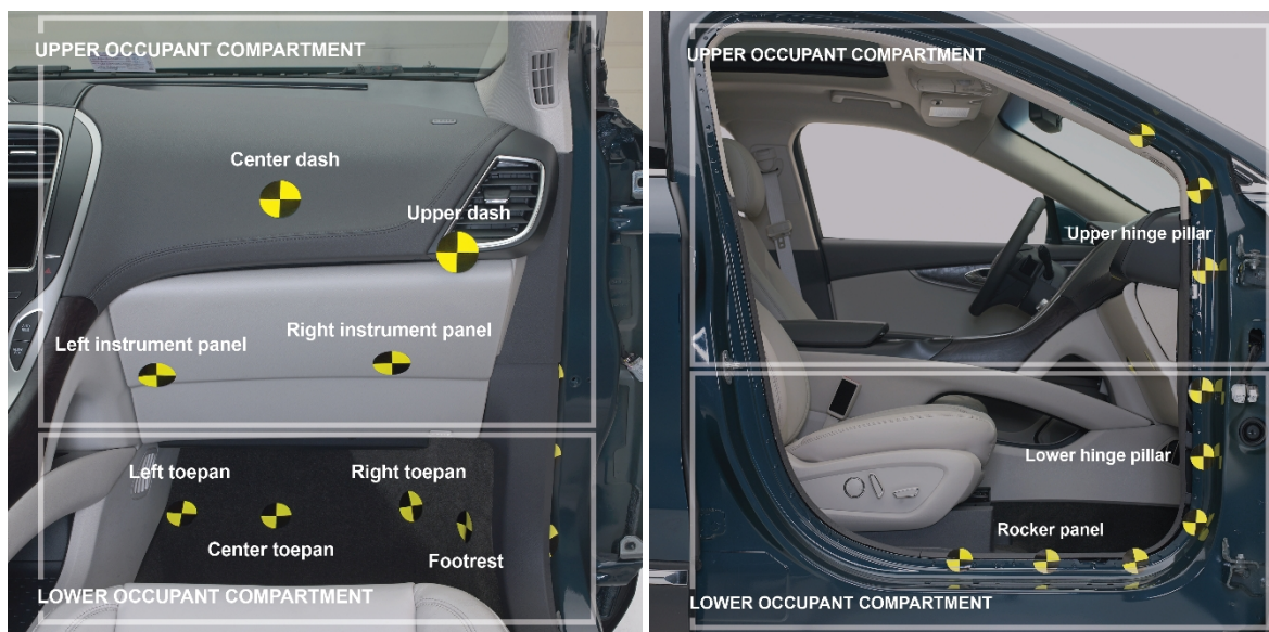
Figure E-2 Locations for Measuring Vehicle Intrusion – Right side
