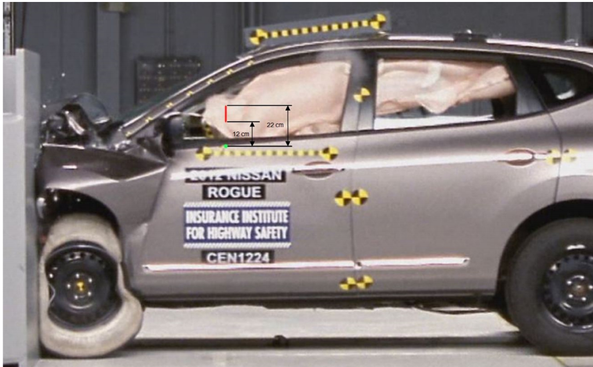
Figure B-4 Steering Wheel Center to Front of Side Curtain Airbag Chamber Measure
