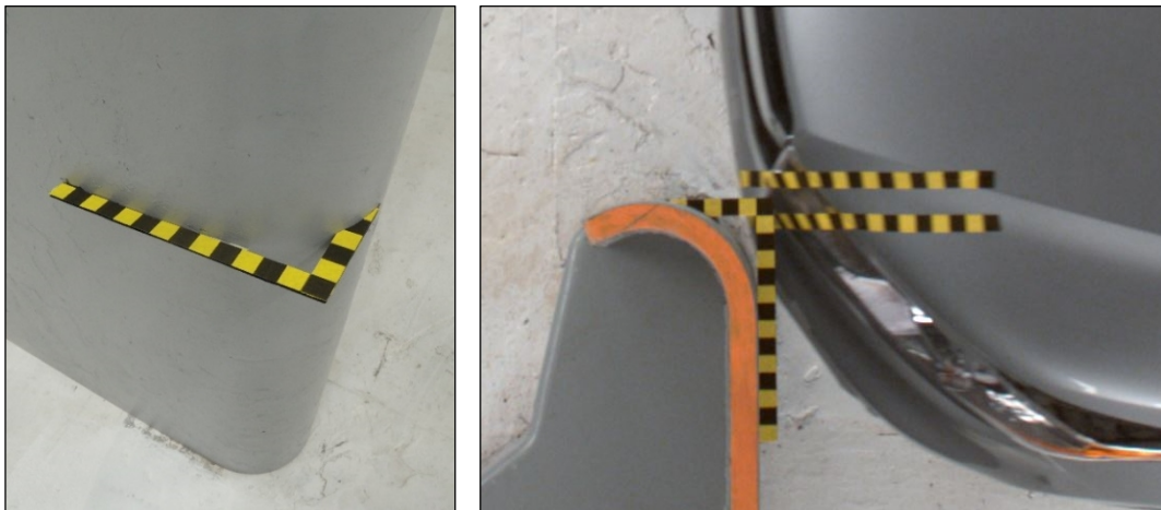
Figure 6 Determining Vehicle Overlap – Target (left) and Video Screen Shot (right)
