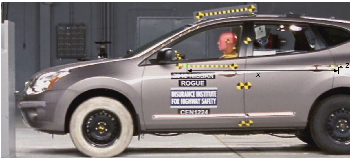
Figure B-1 Rear Door Latch Target to Steering Wheel Center Target Measure
